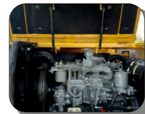
Engine Oil Level Check-up Access
