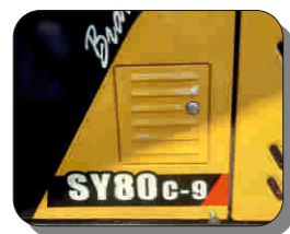
AC Filter Location
