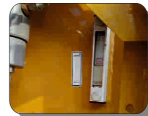
Hydraulic Oil Level Check-up Access
