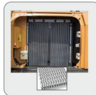
Independent oil cooler & radiator
