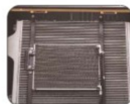
Independent roc with wire mesh guard
