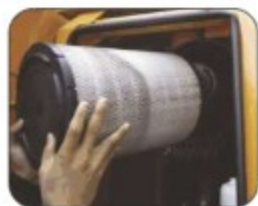
Wire mesh protected air filter
