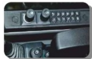
Jog dial & CAN type control switches.
